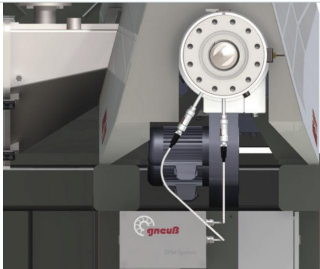
**Fig. 1. The Extruder Pressure Monitoring (EPM) system uses two redundant sensors**
