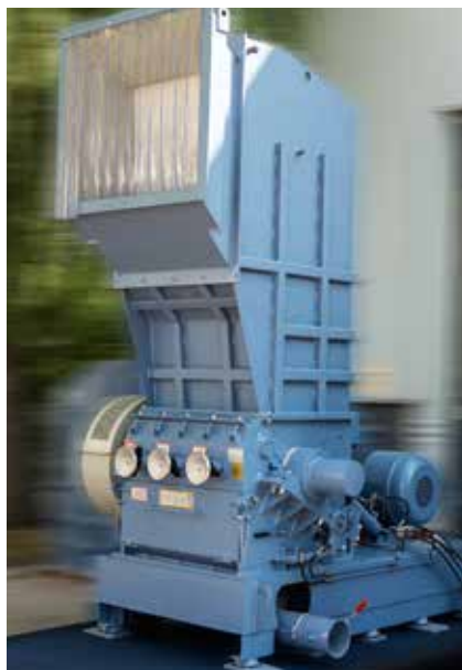
Fig. 4. Cutting mill for preliminary size reduction (figure: Herbold Meckesheim)
