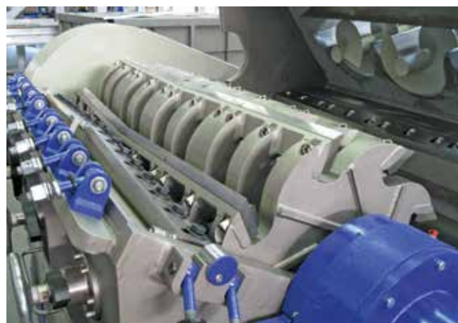
Fig. 5. Cutting mill rotor (figure: Herbold Meckesheim)
