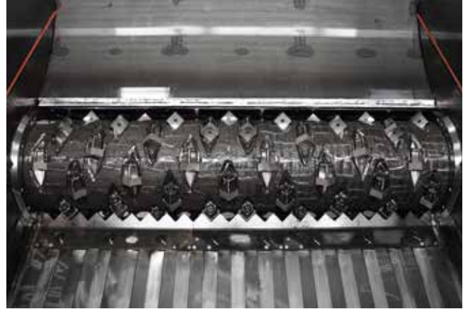
Fig. 3. Shredder rotor: F-Rotor with welded Vautid wear protection (figure: Weima)
