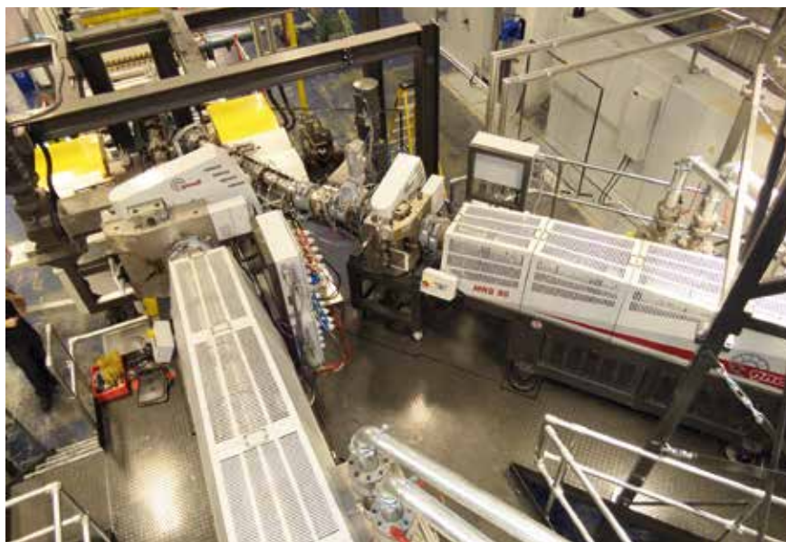
Fig. 3. Integration of a coextrusion line into an existing sheet downstream section (© Gneuss)
